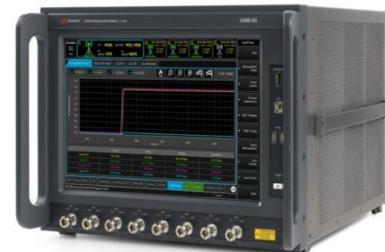
The Keysight UXM 5G wireless test platform is a highly-integrated signaling test platform with multi-format stack support, robust processing power, and abundant RF resources. The UXM 5G wireless test platform enables you to establish a 5G call with a device under test (DUT) in different 5G New Radio (NR) deployment modes, frequency bands (FR1 and FR2), and cellular network configurations.
